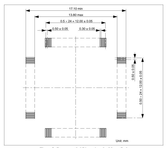
Figure 5 Recommended Dimensions for Mount Pad
